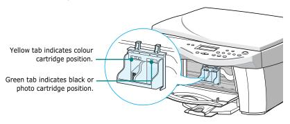
Place the colour print cartridge into the left side of the holder.
